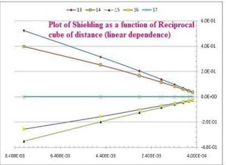
Since it is merely a secondary field without any specific orbital interactions (for energy considerations), these QM results must be the same as the Classical dipole model where the Magnetic dipole is placed at the ring center of optimized benzene.
