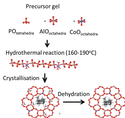
Fig. 5 A schematic illustration of the formation of CoAlPO-5 based on our combined X-ray absorption spectroscopy at the Co K-edge and X-ray diffraction studies reported here and elsewhere. Co(II) = blue, P(v) = orange, Al(III) = light pink, O = red, H = white. The organic template is shown in grey scale.
